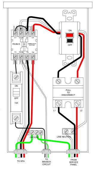
NEUTRAL WIRE FOR 15 AMP BRANCH CIRCUIT MUST BE CONNECTED TO THE NEUTRAL LUG OF THE CONTACTOR
